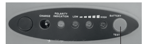
BATTERY CHECK BUTTON
