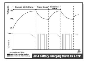
1) Diagnosis & Bulk Charge: As soon charging instruction is given to the charger, the unique diagnostic function automatically checks status of battery (detects voltage). If a battery's voltage is over 3.75V (for 6V battery) or 7.5V (for 12V battery), charger begins fast charging mode by applying a constant current 750mA for both 6V or 12V battery, which terminates when voltage reaches 7.2V (for 6V battery) or 14.4V (for 12V battery).
