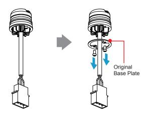
2. Secure Flange Plate to lighthead base with screws.
